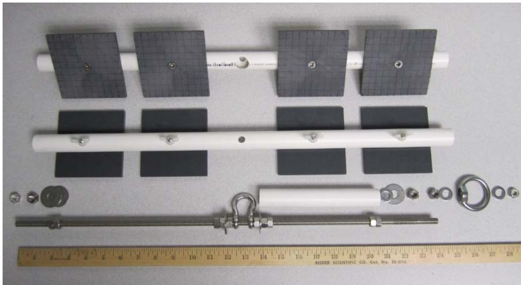
9. Insert the 6-3/4" PVC standoff over end #2 of the threaded rod until it presses firmly against the 1-1/4" OD flat washer added in step 7. The PVC standoff should fit tightly over the 13/16" OD flat washer also added in step 7.
