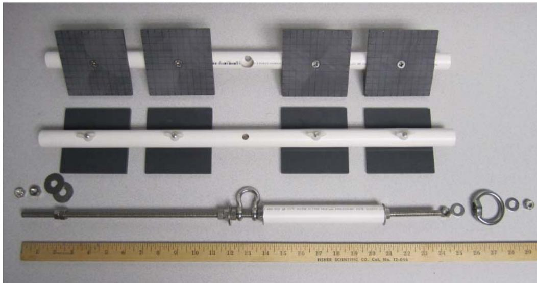
12. Beginning with the 24" PVC section having the 3/4" hole, slide end #2 of the threaded rod through the center hole of the PVC section ensuring that the 3/4" hole and settlement trays are facing end #2 of the threaded rod. Install the second 24" PVC section in a similar fashion perpendicular to the first section added.
